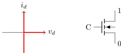
Note: The MOSFET is normally operated with  $i \geq 0$
