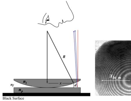
Let  $d$  be the thickness of the space between the two dielectrics, the relationship between  $x$ ,  $d$  and  $R$  is:
