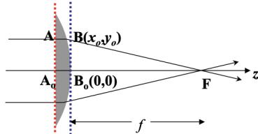
Consider a plane wave incident on a convex lens and focuses to the point  $F$ . As the incident wave is a plane wave, the phase anywhere on the transverse plane just before the lens (indicated by the red line) is the same. From geometric optics, we also know that the OPL for the ray going from  $A$  to  $F$  is the same as the OPL from  $A_o$  to  $F$ .
